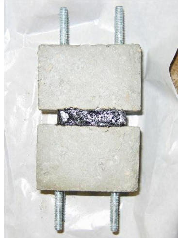
FIGURE 7: Finished product, sealant trimmed and ready for testing
