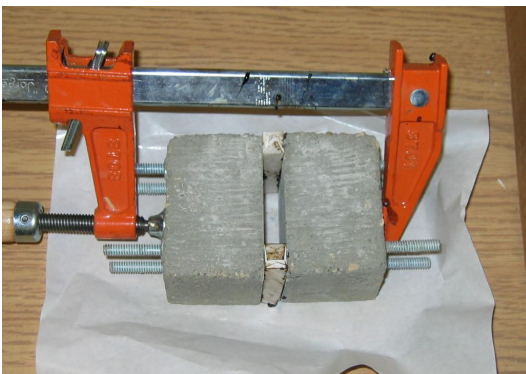
FIGURE 6: Spacers and clamp in place ready for sealant
