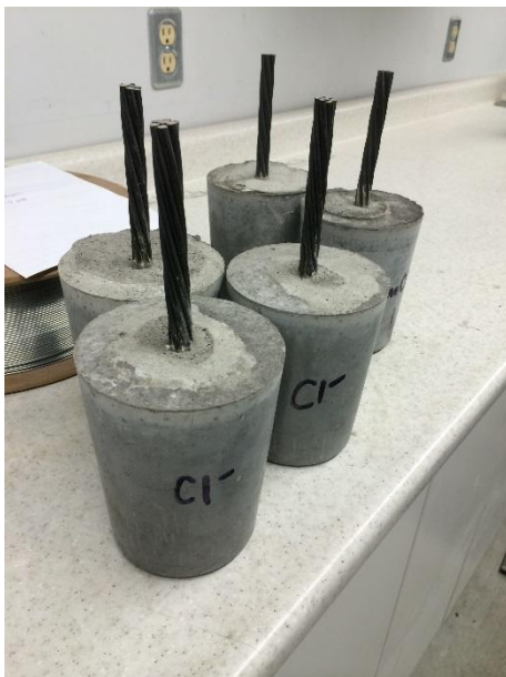
Figure 12. Impregnated and untreated samples prior to potentiostatic testing.
