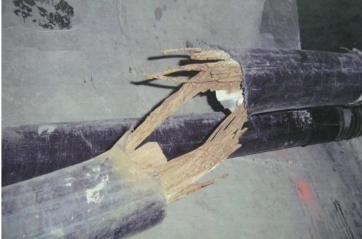
Figure 3. Failed tendon due to corrosion at interface between original Portland cement grout and new grout in re-grouted voids (Virginia Department of Transportation)
