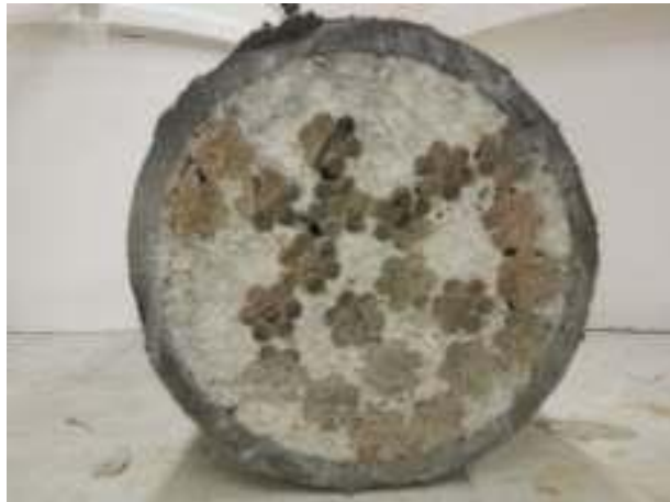
Figure 15. End view of one FDOT tendon specimen as received.
