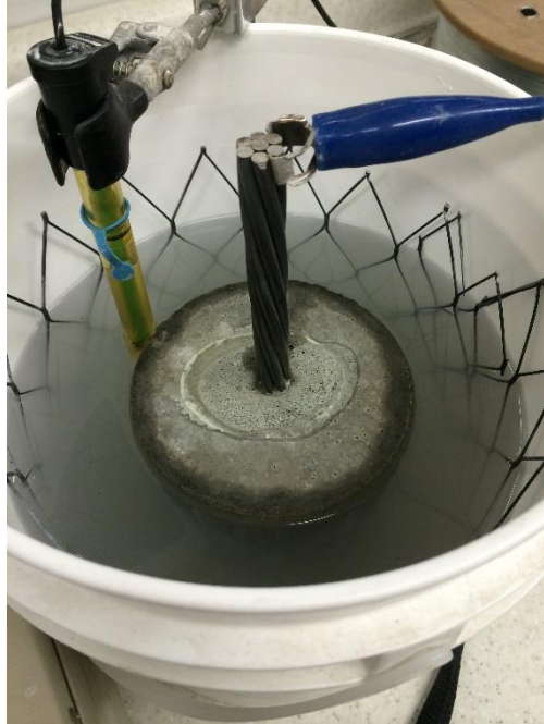
Figure 13. A sample undergoing potentiostatic testing.
