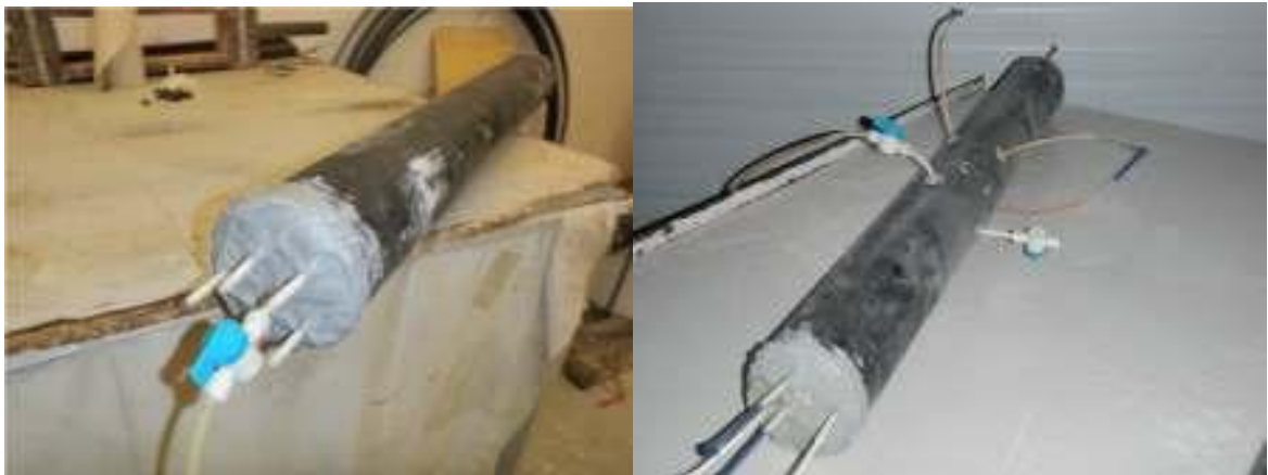
Figure 16. (Left) Impregnation being completed from the end of a prepared specimen. (Right) Impregnation being completed from the midpoint of a specimen.
