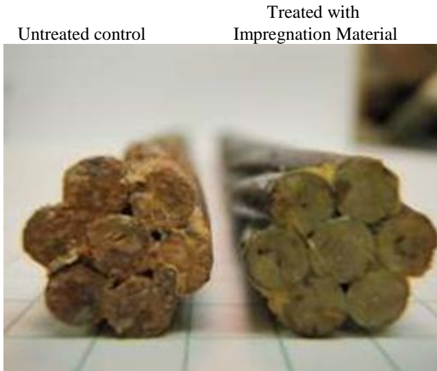
Figure 11. Post-tension strand after exposure to salt spray test.
