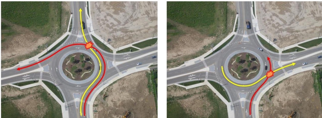
Figure 1.1 Common Crash Types at Multi-Lane Roundabouts
