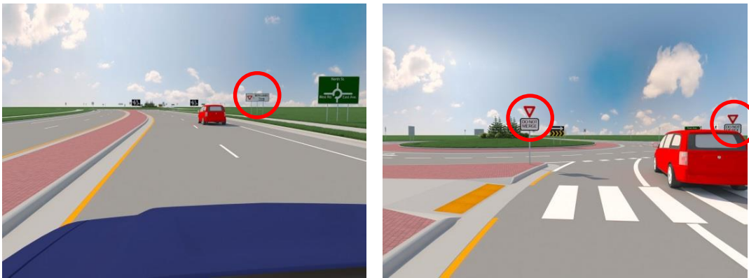
Figure 3.2 Slides Showing the “Yield to Both Lanes” Sign and “Do Not Merge” Tabs
