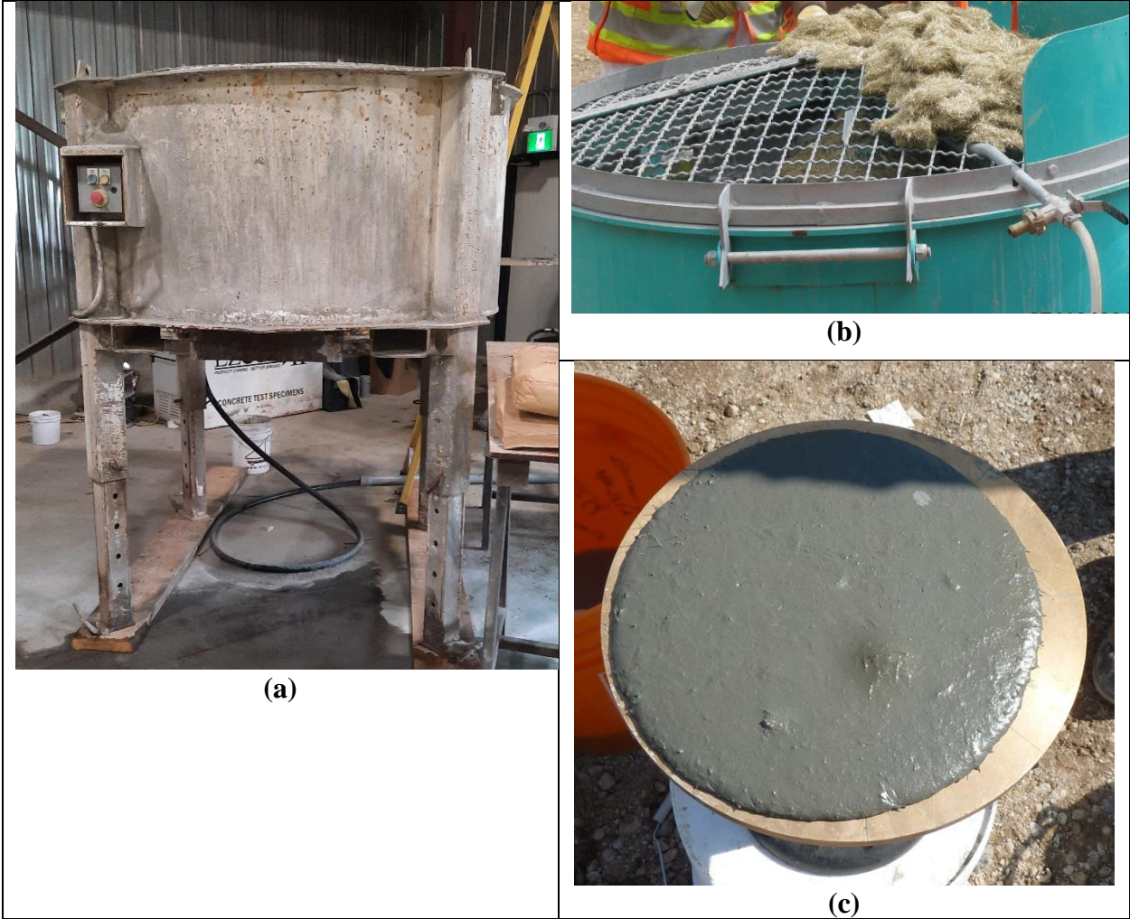
Figure 5: UHPFRC Mixing (a) Typical High Shear Mixer, (b) Adding Steel Fibres (c) Flow Test
