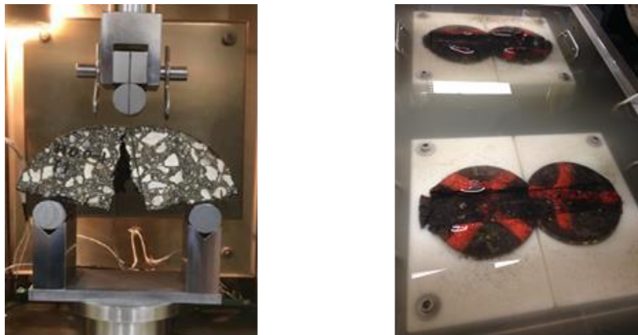
Figure 4: I-FIT (left) and HWTT (right) specimen after testing
