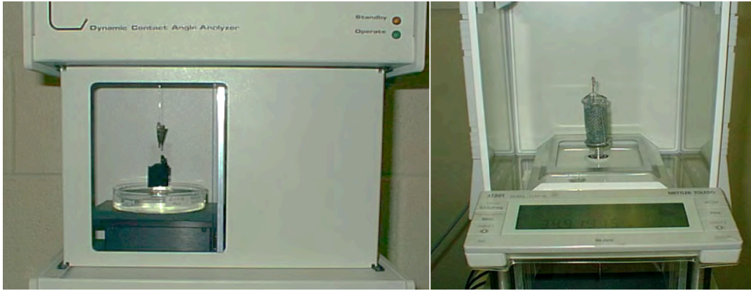
Figure 8. View of Wilhelmy plate and USD apparatus for surface free energy determination
