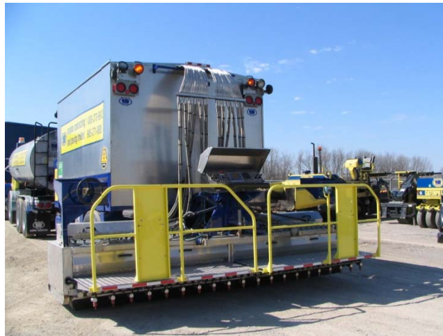
Figure 5. Application deck, showing separate lines of fiberglass capable of up to 4m width in single pass
