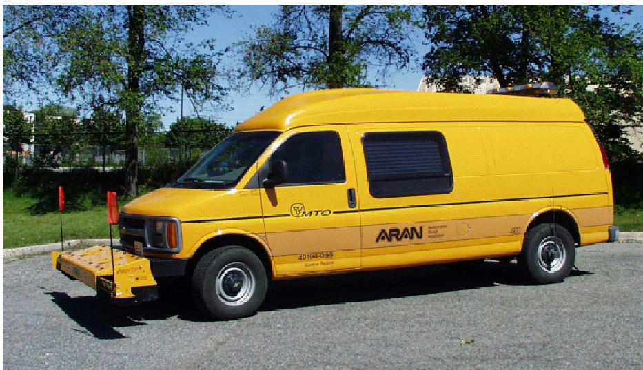
Figure 9. MTO Automatic Road Analyzer (ARAN)
