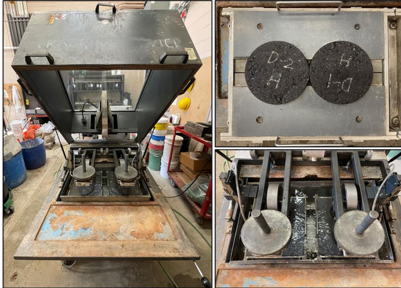
Figure 4: HWT devices, sample moulds, and HWT water submersion
