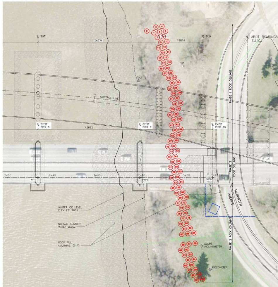
Figure 4 – River Bank Slope Stabilization
