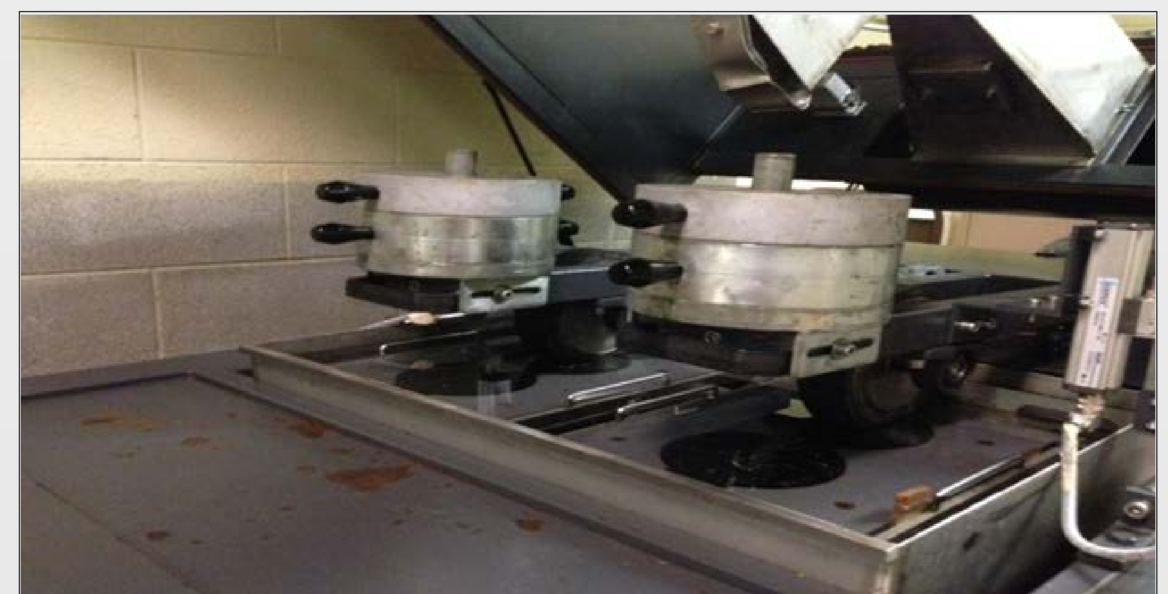
The Hamburg Wheel Tracking Device (HWTd) in accordance with AASHTO T324-04 (2008) is employed to evaluate rutting potential.
