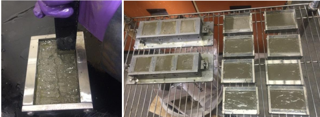
Figure 5. Casting process of a set of mortar coupons and cubes for each aggregate.
