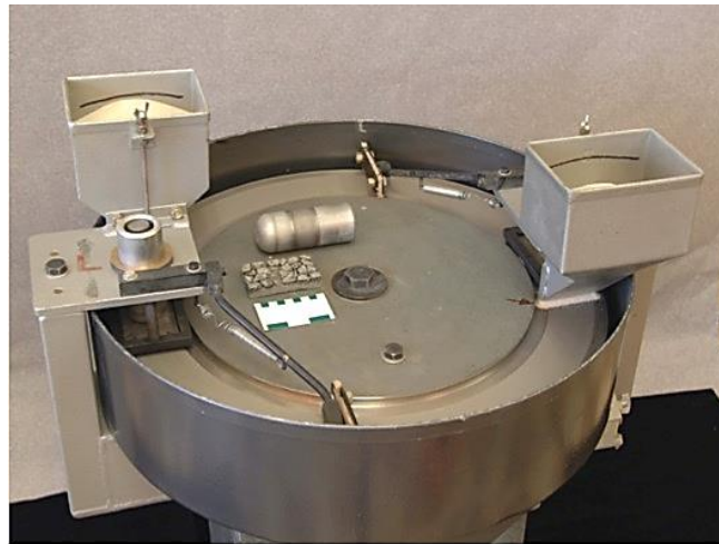
Figure 2. Aggregate Abrasion Value Test Apparatus
