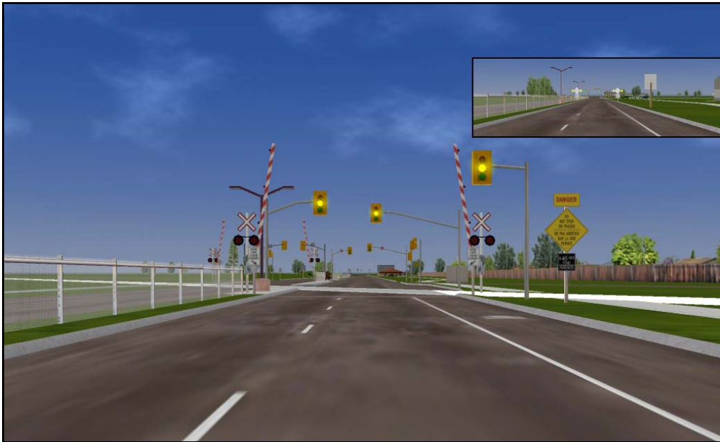
Figure 6: Amber light encountered in dilemma zone while approaching the grade crossing
