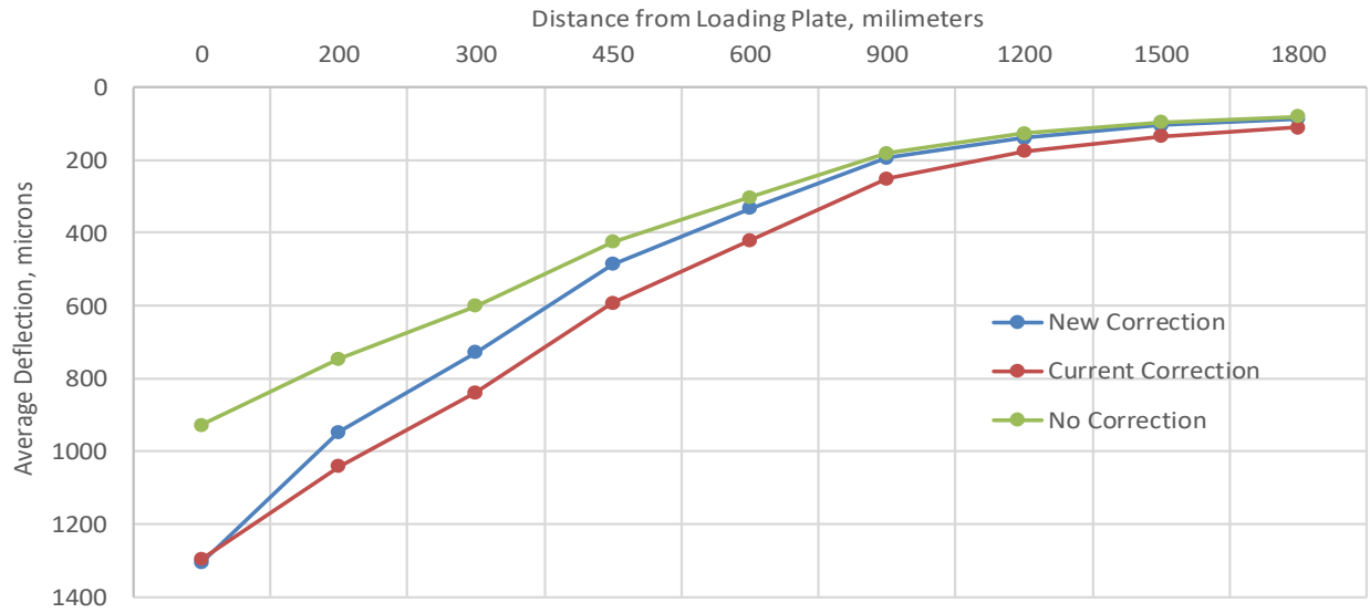
Figure 12. Comparison of deflection basins for PR 352 @ Birnie at 3.6 °C
