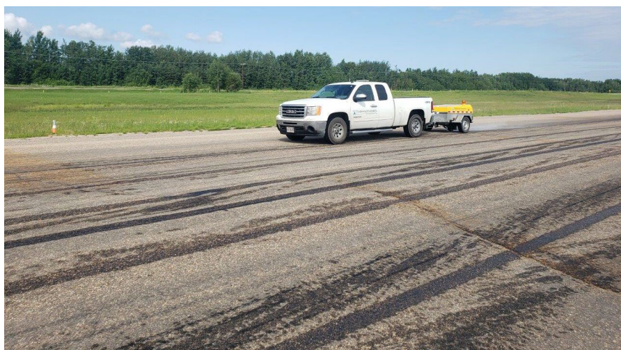
Figure 3 – Surface Friction Testing at Ile-a-la Crosse Airport
