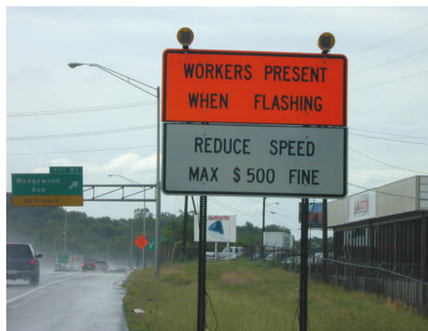
Figure 4. Warning Sign to Reduce Speed when Workers Present (Tennessee) (Source: Ullman et al (81))
