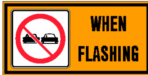
Figure 18. DO NOT PASS WHEN FLASHING Sign (Ontario, Pilot Vehicles and Pace Vehicles) (Source: Ontario Traffic Manual Book 7 (Temporary Conditions)(58))
