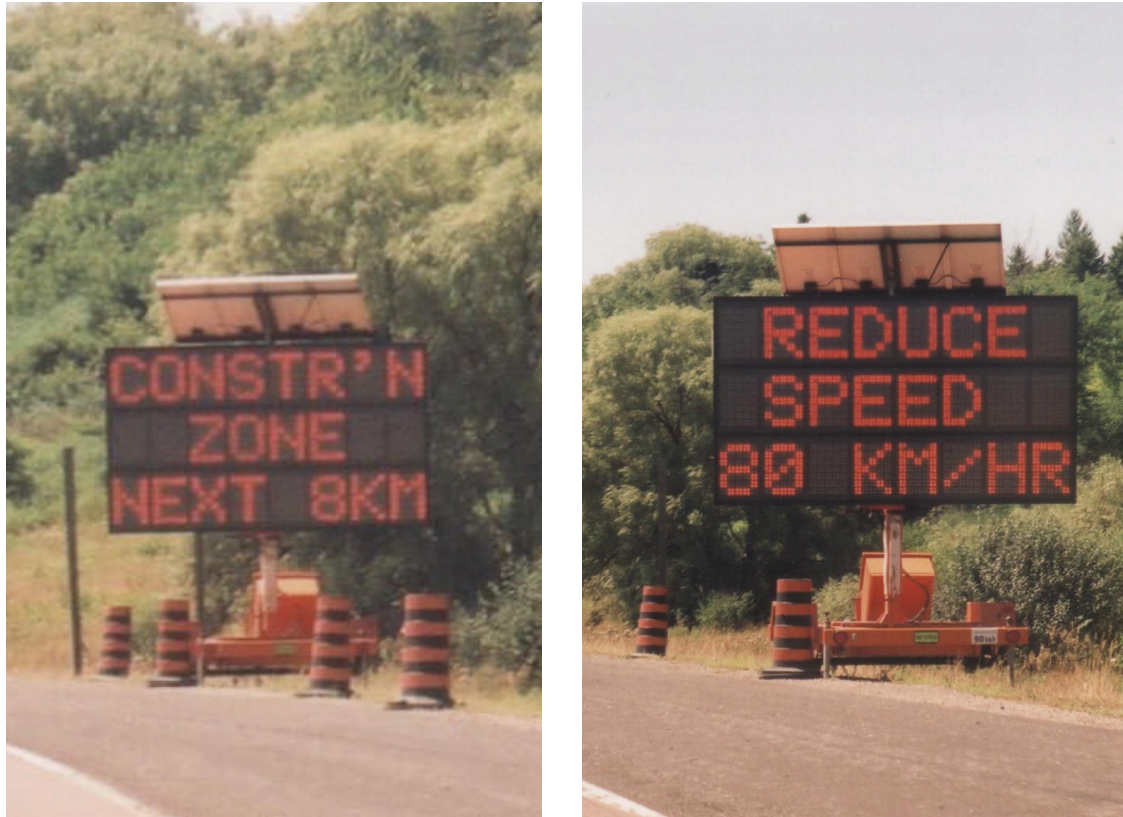
Figure 15. Use of PVMSs for Work Zone Speed Limits (Source: Arges Training & Consulting)
