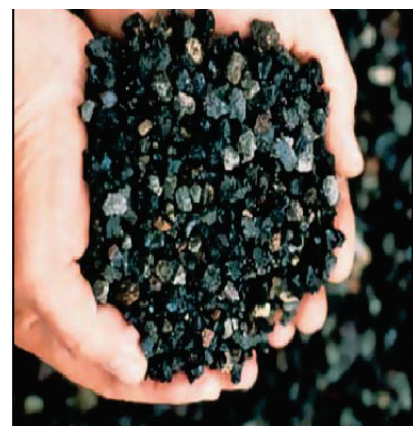
Photograph C3-1 Coal bottom ash in the form of fine aggregate (ACAA, 2011)
