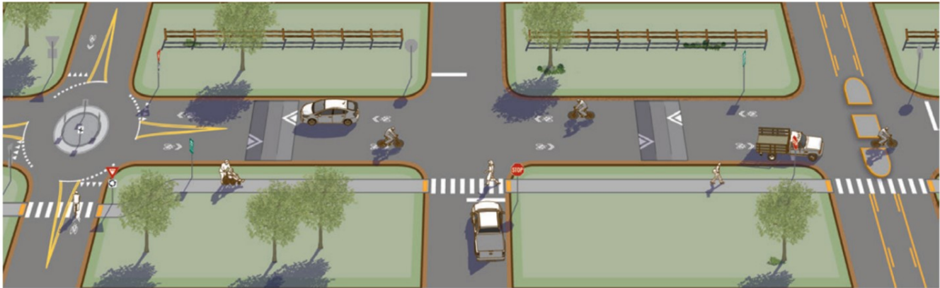
Figure 5: Geometric Design Example of Various Traffic Calming Measures for a Rural or Small Town Bicycle Boulevard (Source: Figure 2-5 in Federal Highway Administration’s 2016 Small Town and Rural Multimodal Networks guide) [89]
