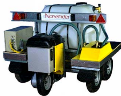
FIGURE 2.5 NORSEMETER ROAR FRICTION MEASUREMENT TRAILER
