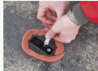
Application of de-icing solution with defined freezing point
