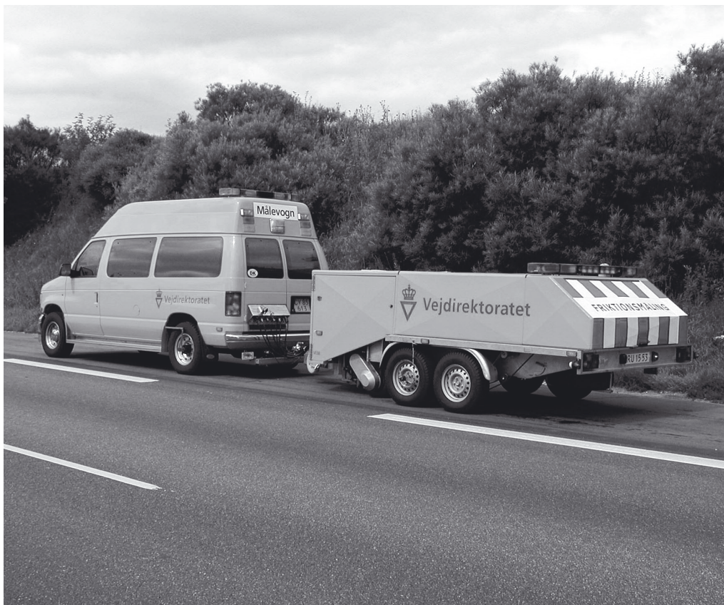
The roughness of the road surface is measured with special lasers, which in turn will indicate the road stretches where roughness is too low.
