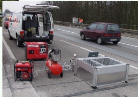
Application of de-icing solution with defined freezing point
