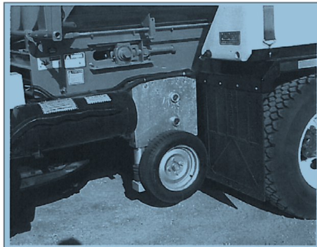
FIGURE 2.7 SALTAR FRICTION MEASURING DEVICE MOUNTED ON A SALTED/PLOW TRUCK
