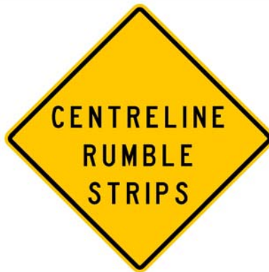
Figure 3: A temporary warning sign used in Alberta in advance of highway section with CLRS to alert drivers to presence of rumble strips along the highway centreline (additional details in Appendix A, Figure 15)
