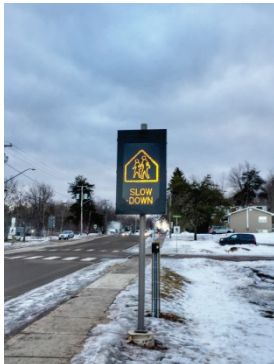
Example of SDD in school zone without speed displayed. Cleveland Avenue, Riverview, NB
