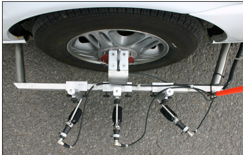
Figure 2 – Arrangement of microphones on the RDA (Uniroyal Tiger Paw All-Season tire; tread depth: 6 mm; tire pressure: 240 kPa)
