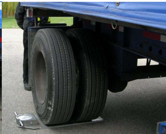
Figure 3 Weighing axle loads on Dual tires
