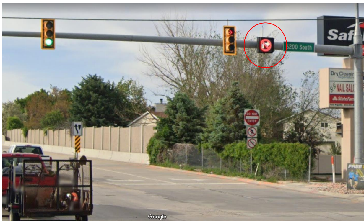
Figure 16: Right-turn blank out signal controlling right turns onto minor roadway
