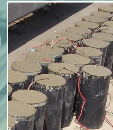
LOGGERS EMBEDDED IN CYLINDERS
