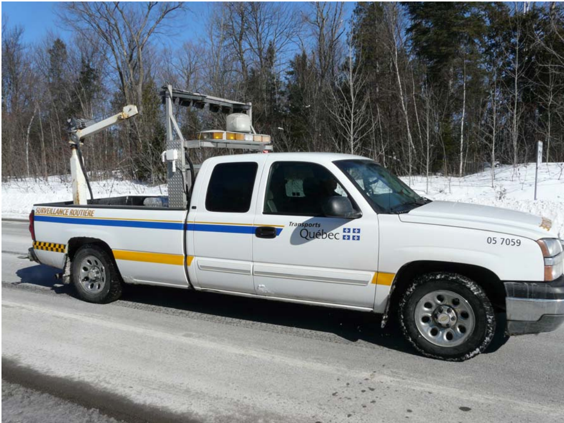
Figure 1: Light-duty truck fitted with a mobile monitoring station
