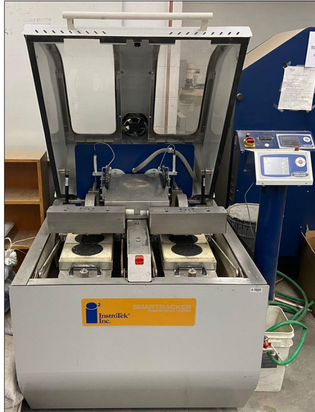
Fig. 7. Hamburg wheel-tracking device and test setup
