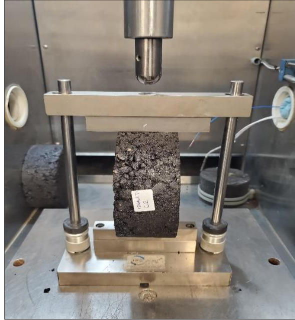
Fig. 6: Indirect tensile strength and IDEAL-CT test setup
