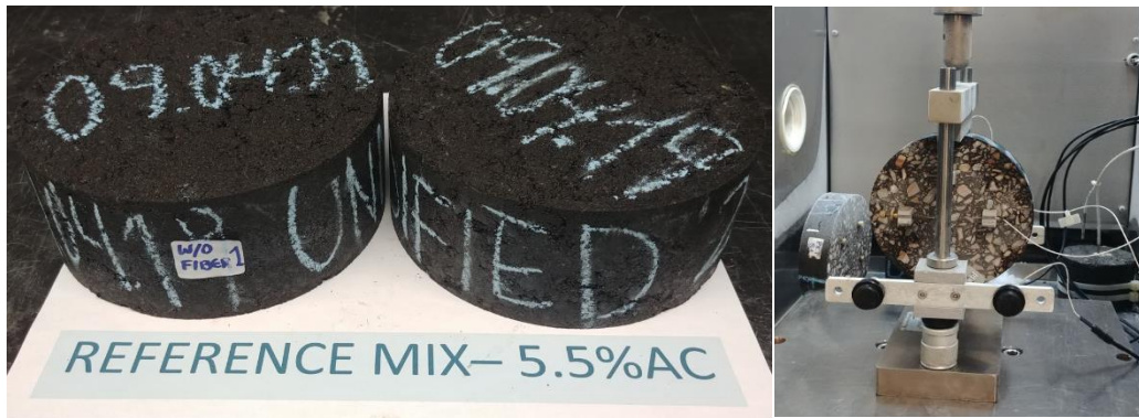
Figure 5: (a) IDT samples, (b) test configuration
