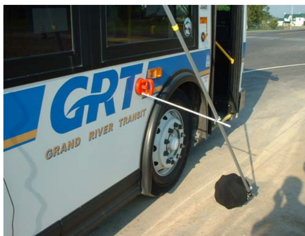
FIGURE 3 – Close-proximity Method Microphone Set-ups
