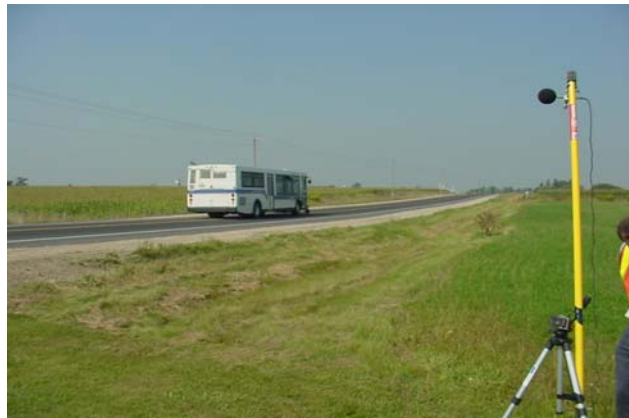
FIGURE 4 – Pass-by Method Monitoring Station Set-ups
