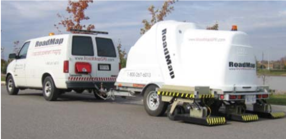
Figure 3: SmartTrailer system with 3 GPR sensors
