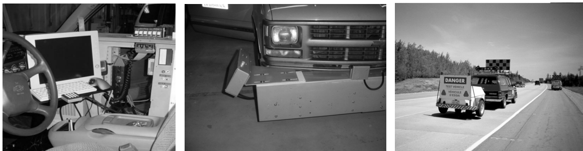
Figure 3: NBDot Data Collection Units – High Speed MDR and Dynaflect Unit
