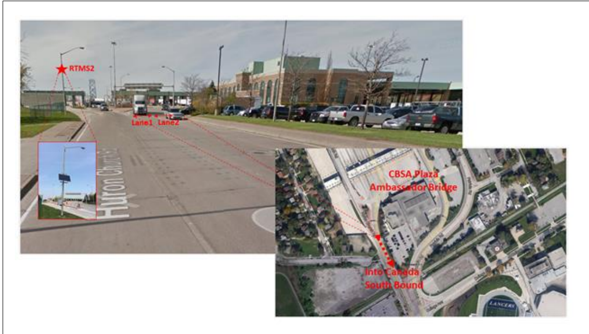
Figure 3. RTMS Monitoring Station at the Exit of the Canadian Custom Plaza at the Ambassador Bridge (Base Image Source: Google Map)
