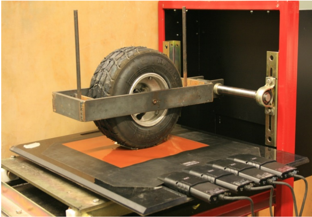
Figure 3. Measurement of test tyre contact patch using a high resolution XSensor pressure pad.
