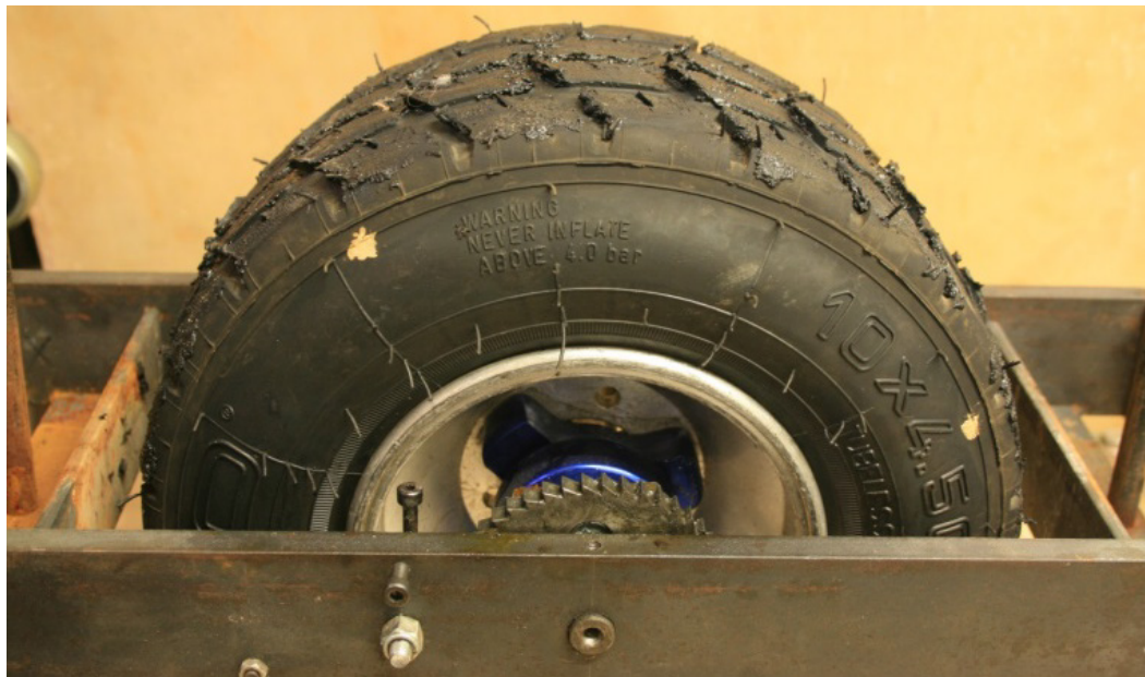
Figure 6. The pneumatic test tyre and braking system.
