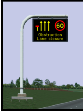
Figure 5 - MM-ALR Verge mounted signalling arrangement
