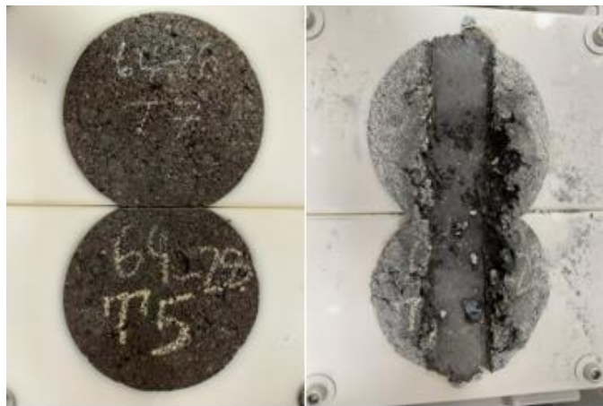
Figure 9: Test Specimens Condition Before and After the HWT Test
