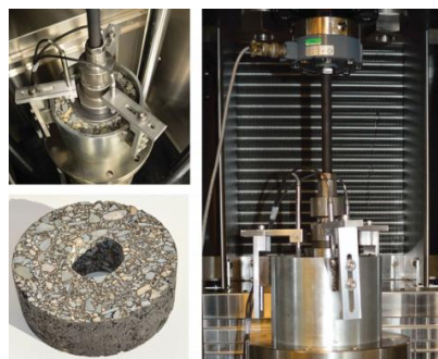
Figure 16: Uniaxial Shear Tester (top view, hollow cylindrical specimen, UST placed in UTM Chamber (Zak et al., 2017)
