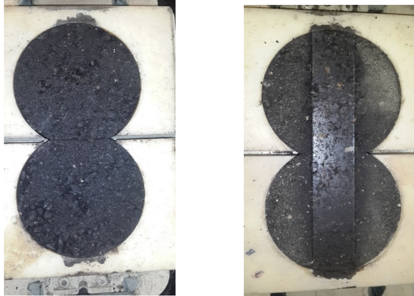
Figure 8: HWTd Cylindrical specimens (saw-cut) in HDPE moulds before (left) and after (right) test
