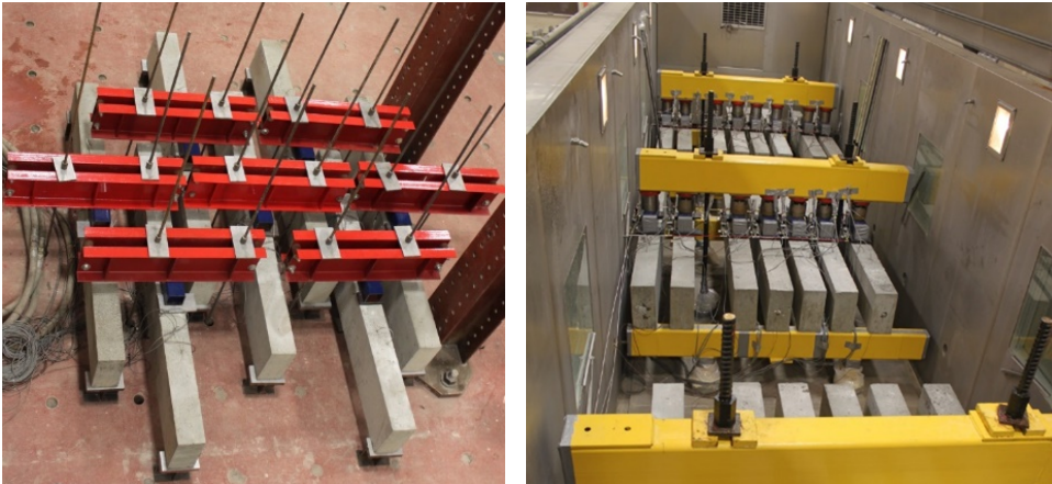
Figure 3: Sustained load applied on control beams and beams placed in the climate chamber
