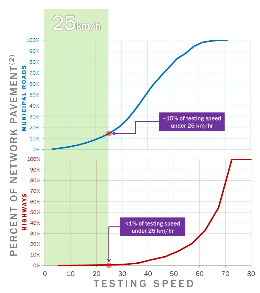
As seen above<sup>(2)</sup>, municipal road pavement networks are significantly affected (~15%) by low speed testing while highway pavement networks are not (<1%). Knowledge of the percent of network pavement affected by testing speed will help determine the course of action used when reviewing and reprocessing invalid IRI data.
