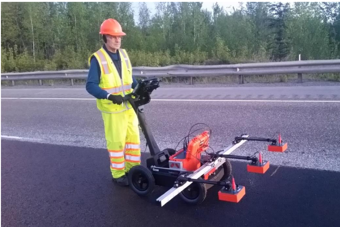
Figure 6 PaveScan Unit measuring Joint and Mainlane Percent Compaction [13]
