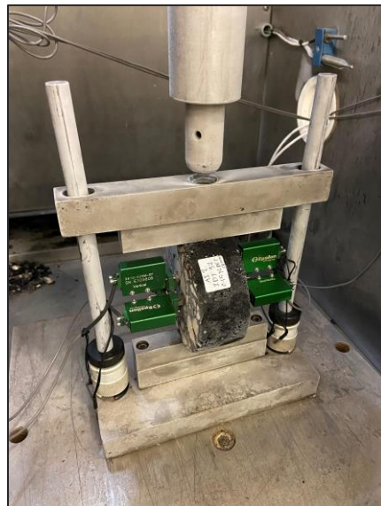
Figure 6: IDT strength test setup
