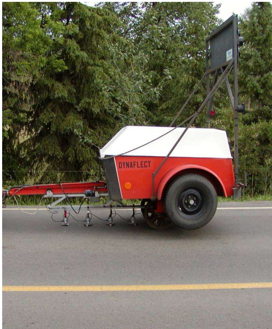
Figure 13 - Dynaflect Deflection Apparatus
