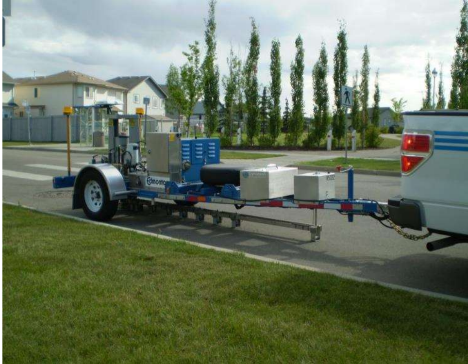
Figure 14 - FWD Deflection Apparatus
