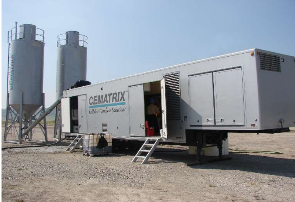
Figure 4 – Lightweight Cellular Concrete Dry Mix Equipment
