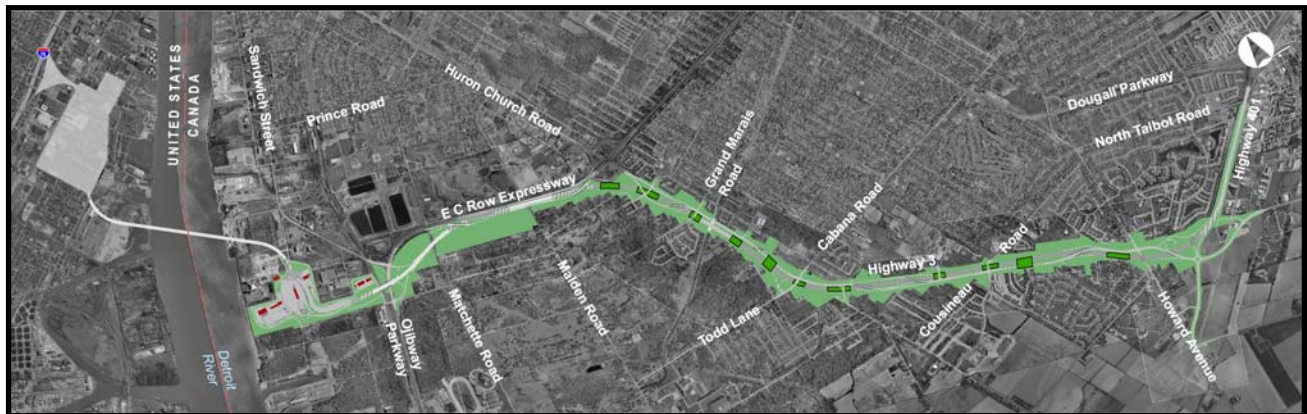
Figure VI: Approved Plan including (L-R) U.S. Interstate Connection, U.S. Customs Plaza, Detroit River Bridge Crossing, Canadian Customs Plaza, Canadian Access Road connection to Highway 401
