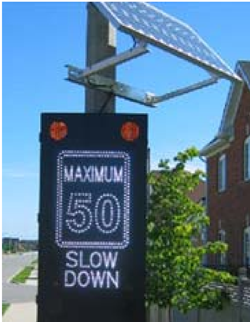
Figure 1: Typical example of iSLOWS used in Calgary
