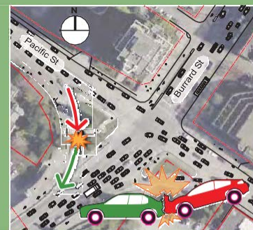
Eastbound drivers turning right from Pacific onto the bridge and rear-ending other vehicles in the slip lane
