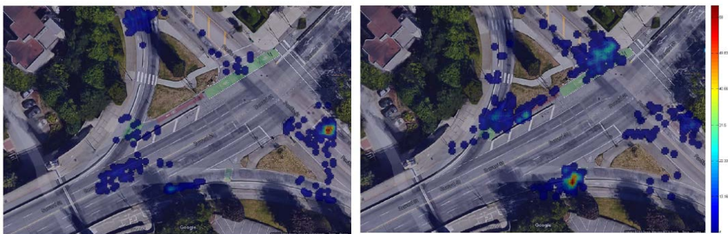
Vehicle-vehicle (left) and vehicle-pedestrian/cyclist conflict frequency heat map Source: Bigazzi, A., Puscar, F., Safed, T., & Zaki, M. (2016). Intersection Safety Diagnosis Using Automated Video Analysis.
