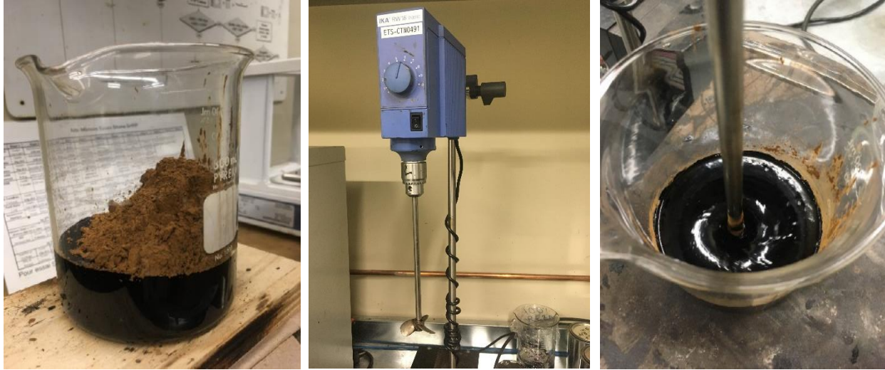
Figure 2. Mixing lignin into bitumen using a conventional asphalt mixer (Carret et al. 2021).
