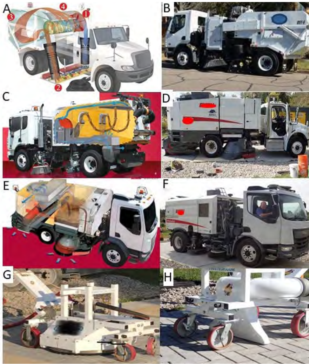
Figure 3-6: Street sweepers (A, B) Tymco® DST 6 regenerative air (Tymco Inc., 2019), (C, D) Elgin® Whirlwind vacuum (Elgin Sweeper Co., 2017), (E, F) Elgin® Waterless Eagle mechanical (Elgin Sweeper Co., 2019) and (G, H) Pavetech Typhoon and PaveVac.
