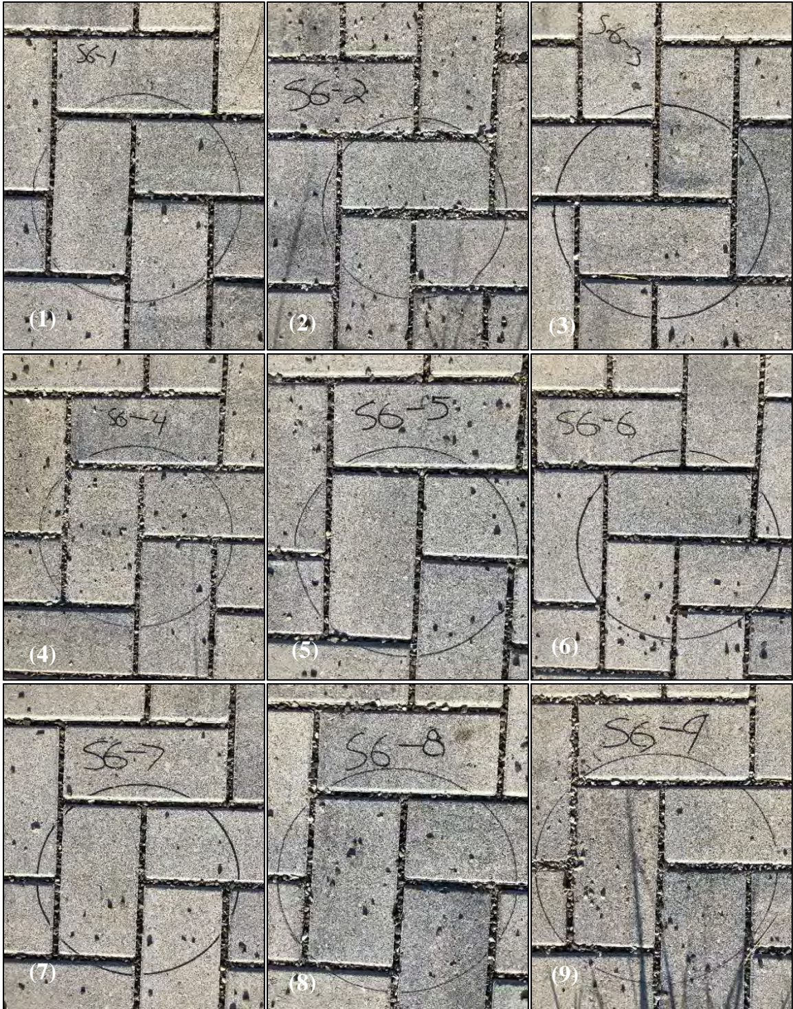
Figure J3. Pre-maintenance photos of infiltration measurement locations (1-9) on Cell 6 after first early and repeated maintenance (TYMCO DST-6®).
