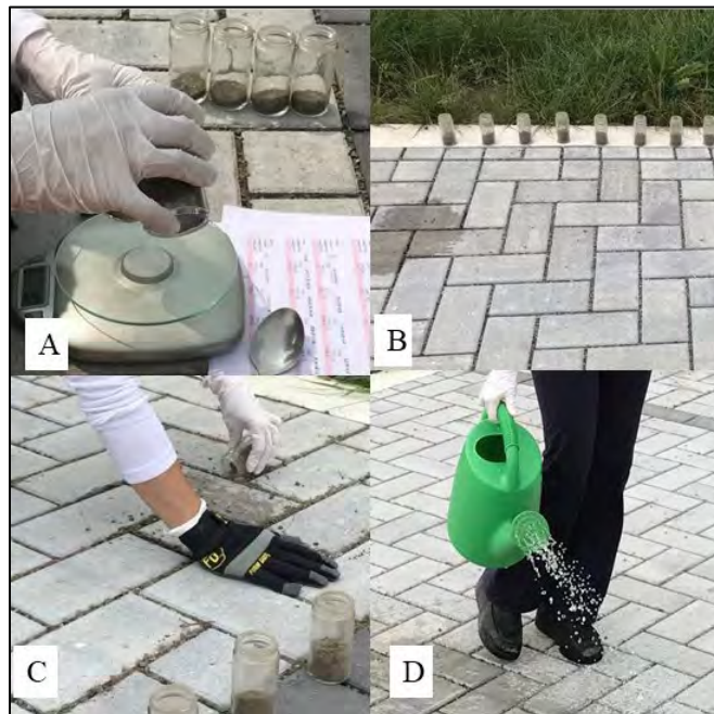
Figure 3-4: Clogging procedure: A) pre-weighing sediment before application; B) pre-weighed sediment for every row and column; C) application of sediment over joints; D) application of water to move sediment into the joints.
