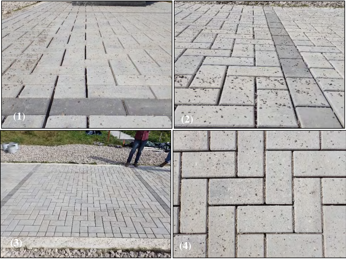
Figure I7. Post maintenance photos following a waterless mechanical sweeper on Cell 5 (Elgin Sweepers Water Less Eagle ® ), where (1) and (2) are parallel and perpendicular to travel path respectively. (3) is an overview of the plot and (4) is a close up of parallel and perpendicular sediment removal.
