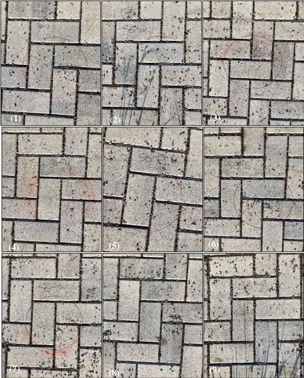
Figure J5. Pre-maintenance photos of infiltration measurement locations (1-9) on Cell 6 after second early and repeated maintenance (TYMCO DST-6®).
