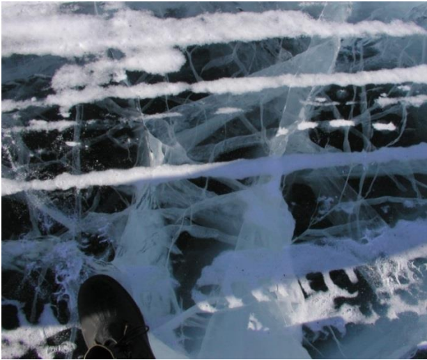
Figure 6: Left) Crack network inside an ice cover (boot for scale) - the crack surfaces are generally vertical, albeit with various orientations. Right) An overnight decrease in air temperature, for instance from -5^{\circ}\text{C} to -20^{\circ}\text{C} as shown here, will induce a tensional regime in the upper part of the ice cover, and result in cracking.
