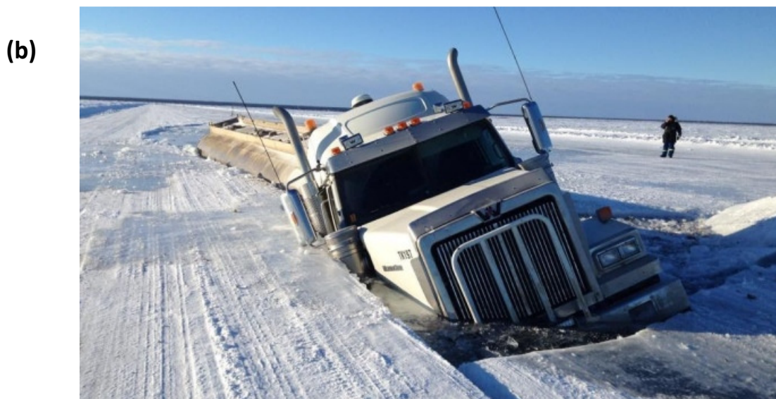
Figure 6. (a) The theoretical normal stresses at the bottom of the ice road along the road for two different ice road thicknesses for the northbound case. Fluctuations in tail regions are integration noise and can be overlooked. (b) A recent, March 2016, incident in an ice road near Deline, NWT happening for a loaded moving truck. The circumstances that led to this incident are unknown to the authors as of this writing. The crack shapes suggest that an along-the-road crack has happened before an across-the-road crack. Picture is courtesy of NWT Environment and Natural Resources.
