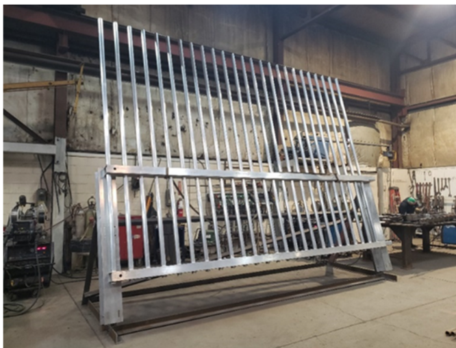
Figure 9 – Mockup of Full-Scale Test Panel
