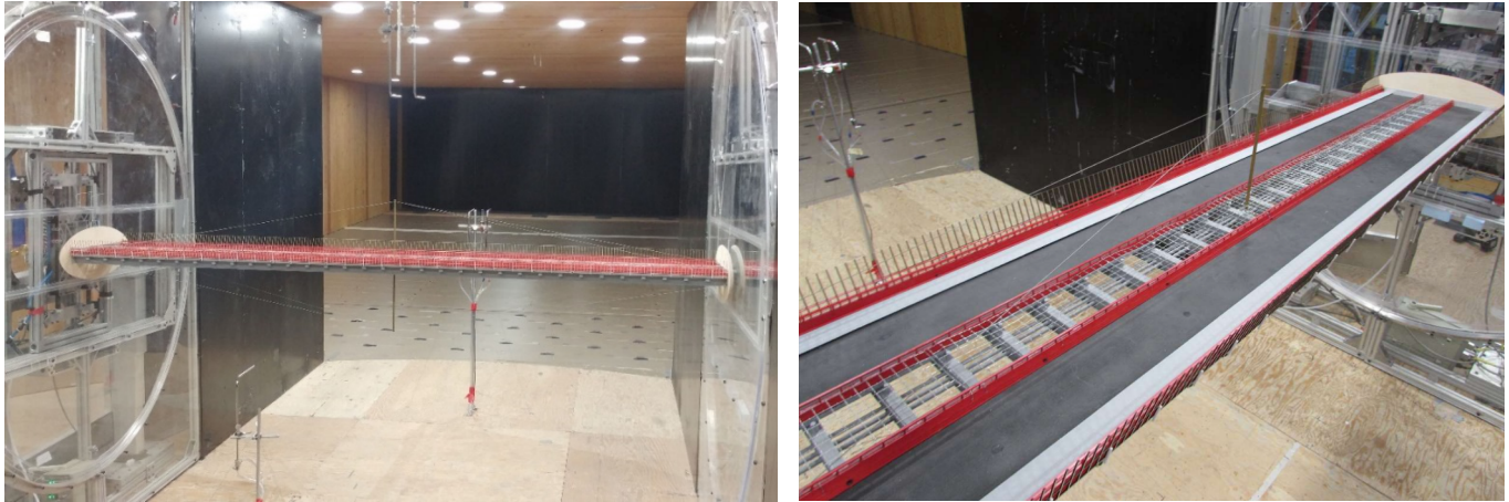
Figure 6 – Bridge Scale Model Wind Tunnel Testing with Barriers
