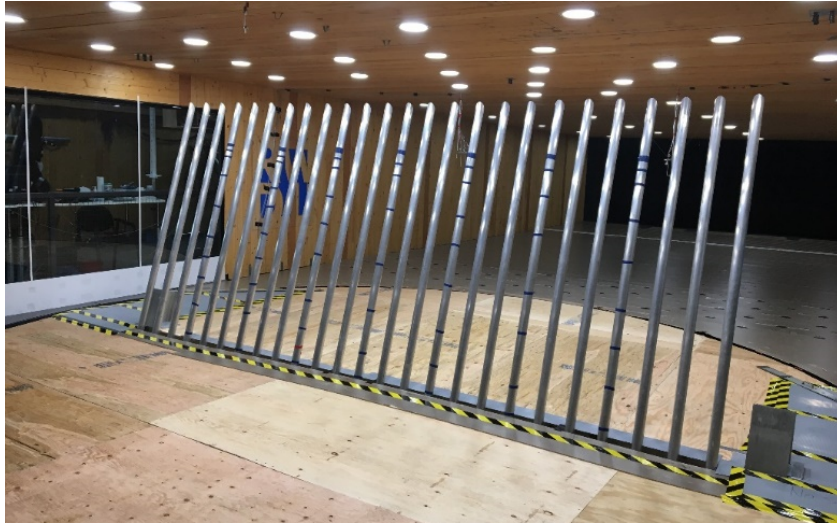
Figure 7 – Panel Wind Tunnel Testing
