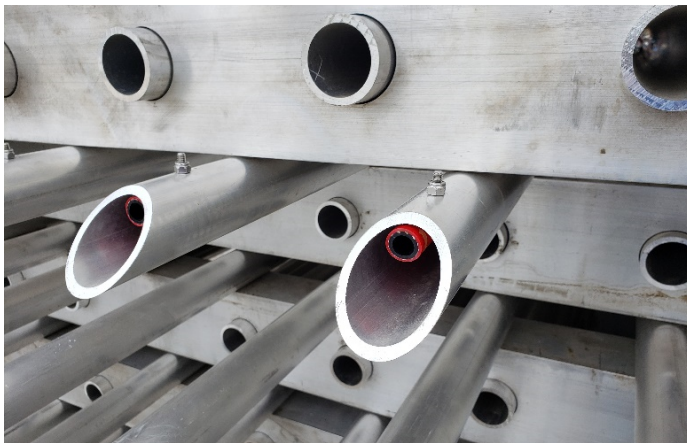
Figure 8 – Pipe Mass Dampers
