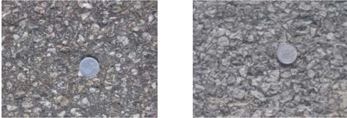
Figure 8. Dense graded HMA (left) and rubberized OGFC (right) at CPATT Test Site
