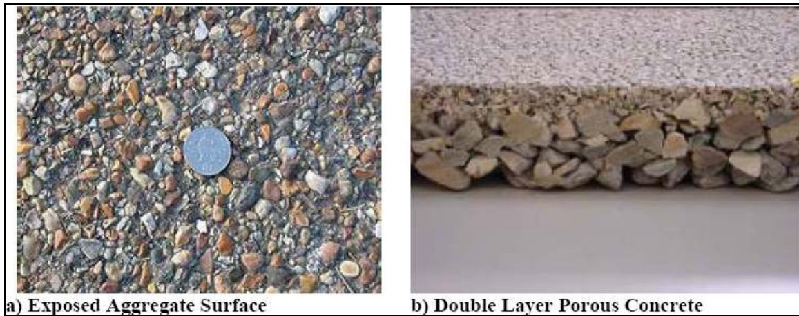
Figure 12. Exposed aggregate and porous concrete surfaces (19).
